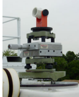
Fig. 3 Translation Stage and Target
