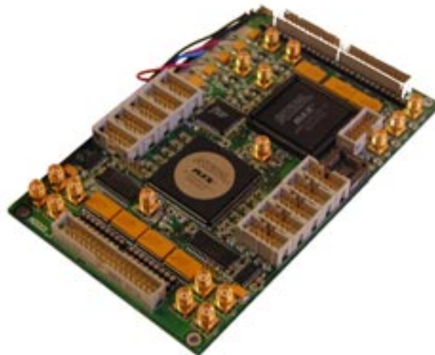
Figure 3 : Digital module. There are 3 programmable cards for the counter, the frequency synthesis control, and the global control.
