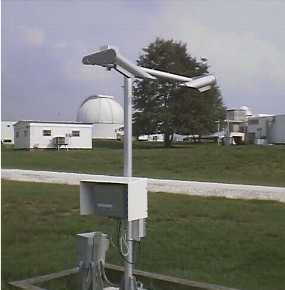
Figure 4. The Vaisala model FD12P. The small box atop the left arm is the DRD12.
