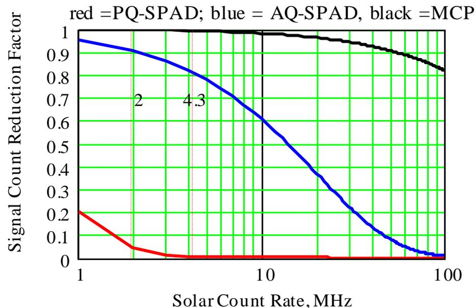
Only MCP/PMTs and Actively-Quenched SPADs (AQ-SPADs) have adequate recovery times for single photon ranging systems. New “silicon photomultipliers” can provide comparable pixellated arrays with 100s to 1000s of small aperture, actively quenched APDs per pixel and **may** have cost, flexibility, and availability advantages as well.
