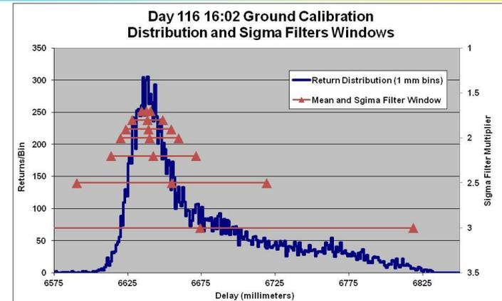
**NGSLR ranging to calibration target with MCP/PMT, 50 psec laser, and HTSI ET (Clarke et al, 18<sup>th</sup> SLR Workshop, Japan)**
