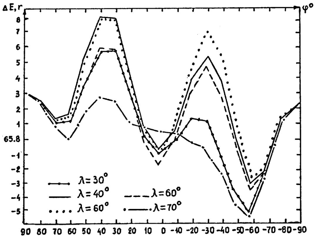
FIG. 13. VARIATION OF ETALON-1,2 REFLECTIVITY AT EACH LONGITUDE
