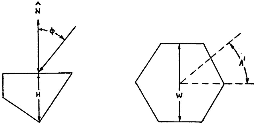
Fig.4. DIRECTION OF INCIDENT BEAM
