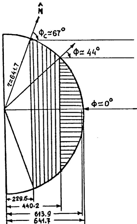
Fig. 9. APPARENT REFLECTION POINTS AND SPREAD IN RANGE
