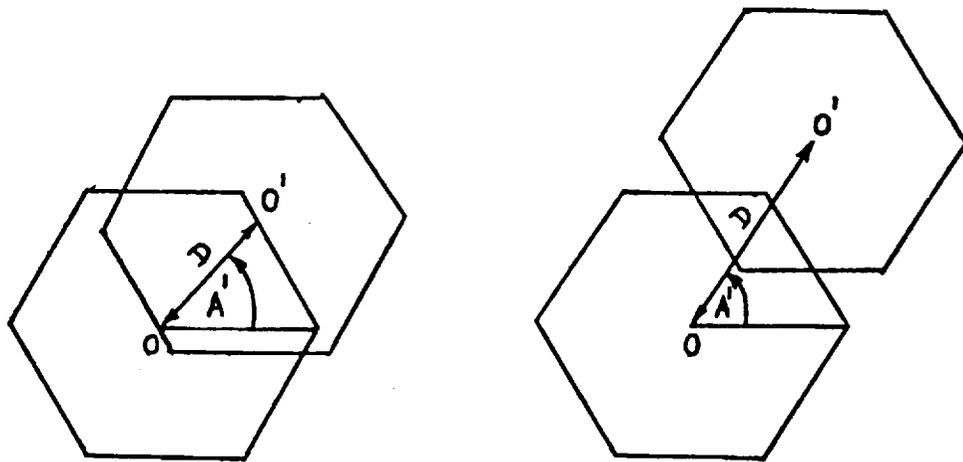
Fig.5. ACTIVE REFLECTING AREA: SEPARATION OF INPUT AND OUTPUT APERTURES
