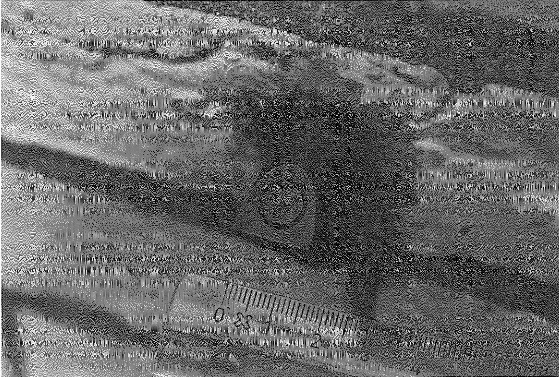
Figure 6 A marker attached to a vertical wall. An engraved circle of 9 mm diameter facilitates pointing the laser beam. The pinhole materializes the actual reference point.
