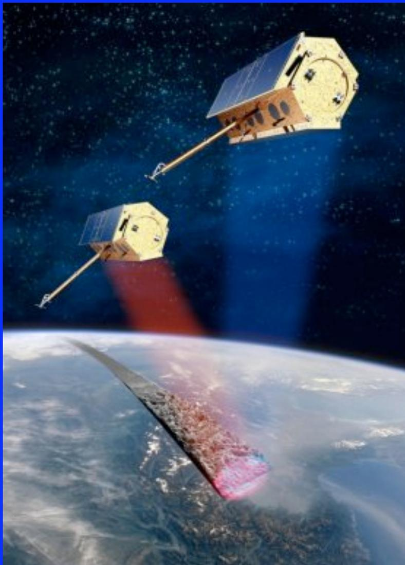
TanDEM-X shall fly in close formation (~300 ... 600 m distance) with TSX to obtain simultaneous X-band radar takes for Digital Elevation Models (DEM)
