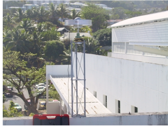
Fig. 14: GPS antenna on the TAHI mark
