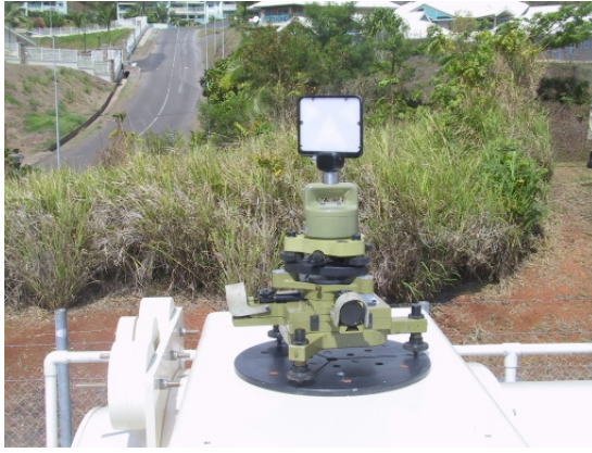
Fig. 11: the translation stage with a target, on the telescope
