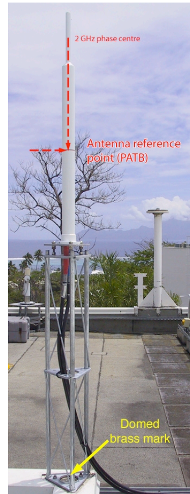
Fig. 5: the DORIS PAQB antenna reference point
