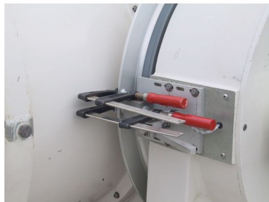
Fig. 10: C-clamps securing the telescope
