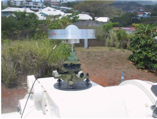
Fig. 13: GPS antenna centred above the SLR telescope
