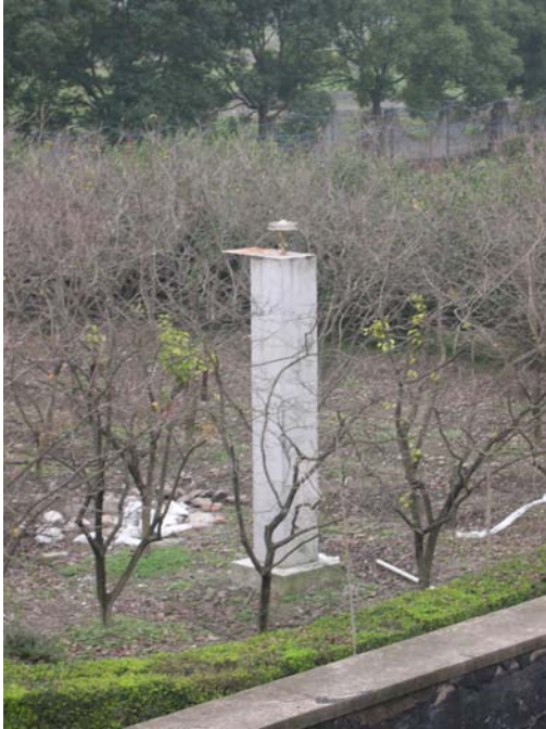
Choke Ring antenna of EGNOS GPS station
