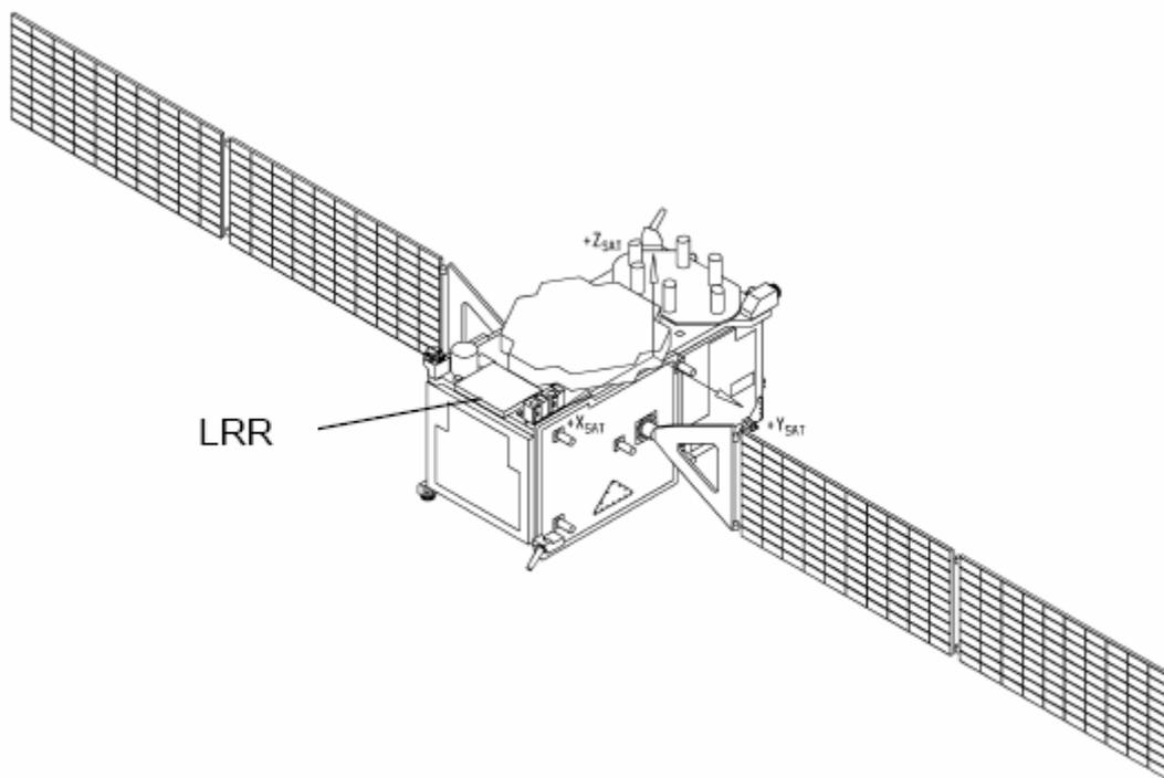
**Fig 3. Position of LRR in a Galileo Satellites.**
