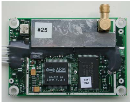
Figure 3. Phoenix GPS receiver board (PROBA-2 engineering model)
