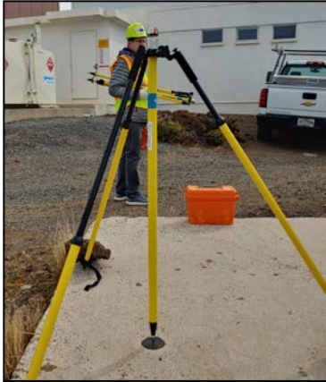
Forced-centering device to occupy a mark
