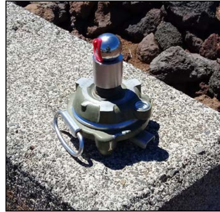
Kern trivet with forced-centering pin
