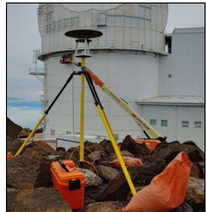
Fixed-height range poles for reflectors and GNSS antennas
