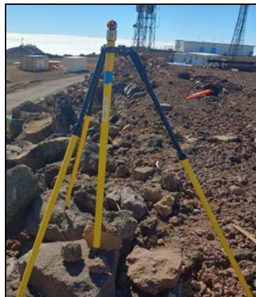
Fixed-height range poles for reflectors and GNSS antennas
