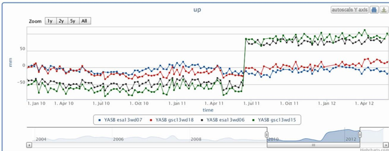
**Fig. 3** Time series of weekly station height determination for Yarra-gadee station: two solutions used for ITRF2008 and their current preliminary solutions for ITRF2013 (using Plottool). Previous esawd08
