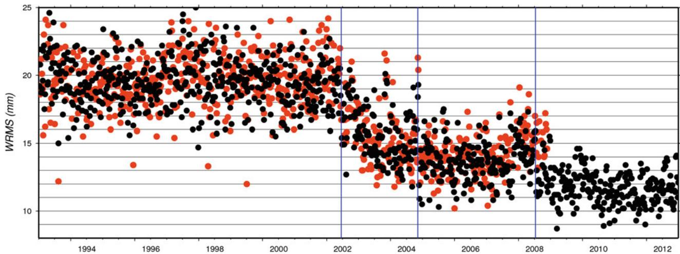
**Fig. 7** Internal consistency of the gscwd10 (previous solution in red) and gscwd23 solution (new solution in black). 3D WRMS when comparing station positions in 3D with the previous week. Vertical lines in blue correspond to changes in the DORIS constellation
