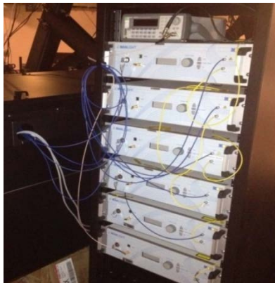
Figure 11 LLOT beacon laser system with six independent fiber based sources mounted in rack near optical bench.
