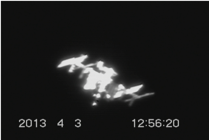
Figure 6 ISS image taken near zenith with telescope blind pointing to a JPL generated ephemeris file
