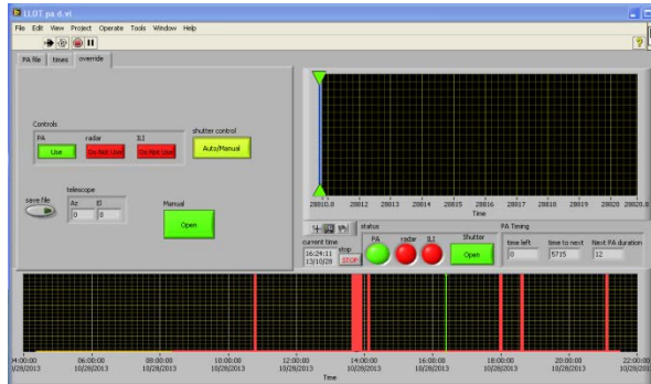
Fig 12 Laser safety control program showing PA outages (red) with shutter controller
