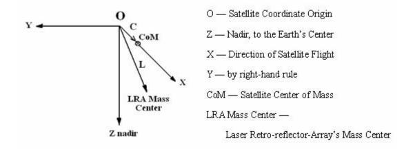
Vector C is from the satellite coordinate origin to the satellite's center of mass (CoM). Vector L is from the satellite coordinate origin to the mass center of the LRA containing 42 corner cubes.
