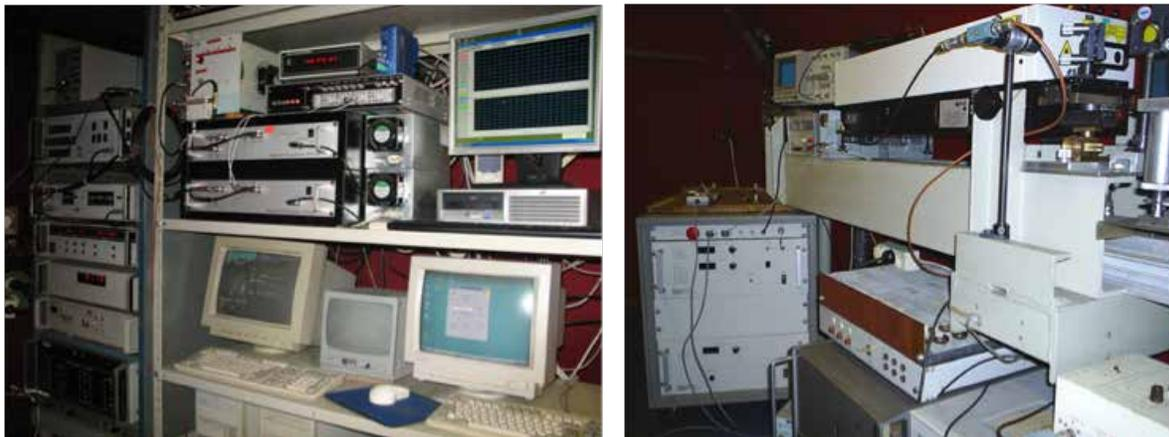
Figure 12-70. Electronics for telescope drive and data registration left; "EKSPLA" Electro-optically Q-switched SBS-compressed Nd:YAG laser SL312 with pulse energy 120 mJ at 532 nm, pulse duration 150 ps (FWHM), pulse duration stability 10%, repetition rate 10 Hz, beam profile Hat Top, diameter 9 mm and divergence <math><0.5\text{ mrad}</math> right.
