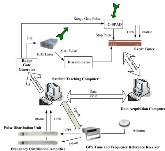
Figure 12-6. The Beijing station's kHz SLR system.
