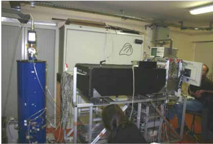
*Figure 12-25. Transportable atomic fountain clock in Grasse developed and installed by the Observatoire de Paris group.*
