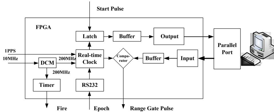
Figure 12-11. Elementary diagram for the range gate generator.
