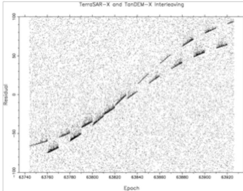
Figure 12-50. SLR returns from TerraSAR-X and TanDEM-X using the interleaving technique.
