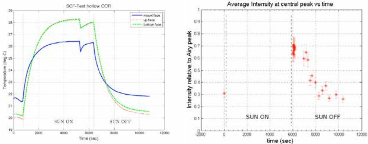
Figure 9-4. (Left) SCF-Test of the Hollow CCR. Drop in temperature at the end of heating phase due to quick turn in front of laser to set up subsequent FFDP acquisition. (Right) Intensity variation of FFDP at the central peak during the SCF-Test. Relative error on intensity is  $\pm 10\%$ .
