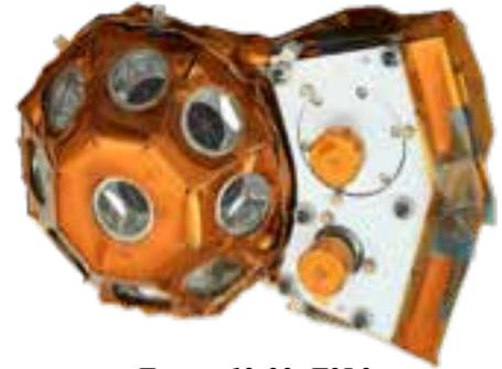
Figure 12-22. T2L2 reflector and receiver.
