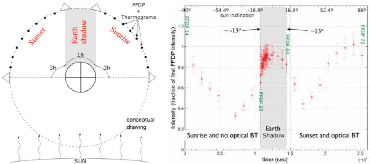
Figure 9-6. (Left) Galileo GCO conceptual drawing. (Right) FFDP average intensity, relative to the first FFDP, of the IOV CCR during the GCO at  $24 \mu\text{rad}$
