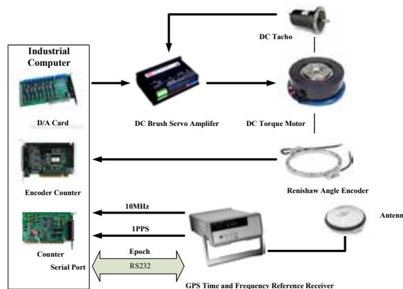
Figure 12-10. Schematic diagram of the servos and encoders.
