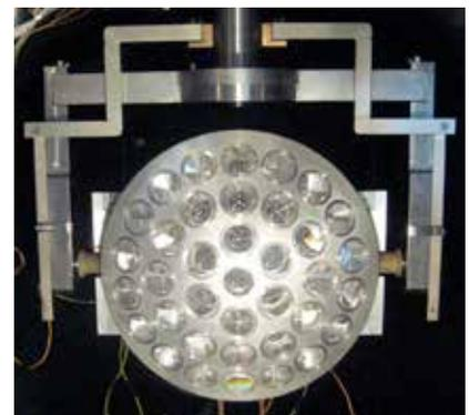
*Figure 9-1. LAGEOS sector inside the SCF cryostat*
