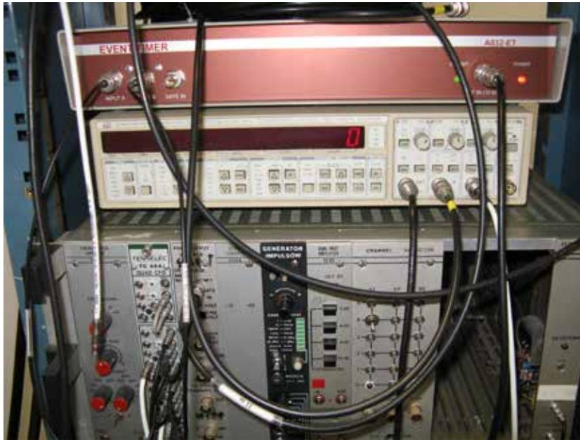
Figure 12-13. Riga Event Timer, below Time Interval Counter “Stanford”.
