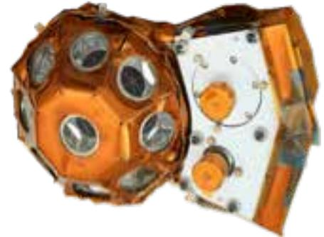
Figure 12-22. T2L2 reflector and receiver.
