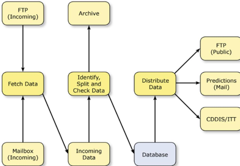
Figure 5-4: Data flow at the EDC
