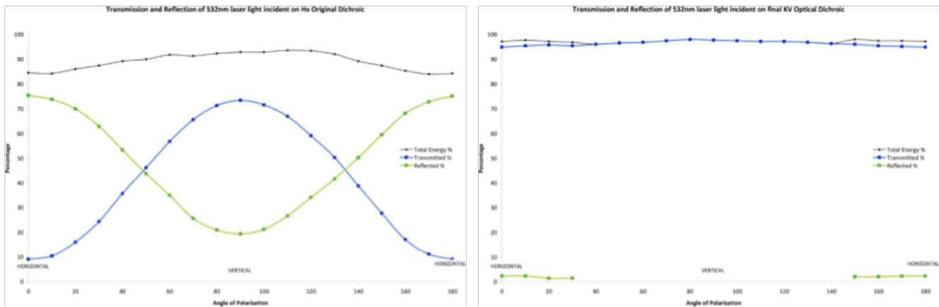
Figure 12-46. The old (left) and new (right) dichroic mirror tests for reflectance dependence on polarisation .
