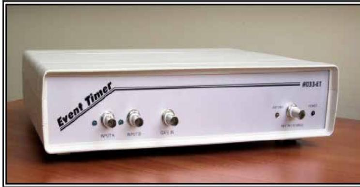
Figure 12-58. A033-ET with  $<5\text{ps}$  precision
