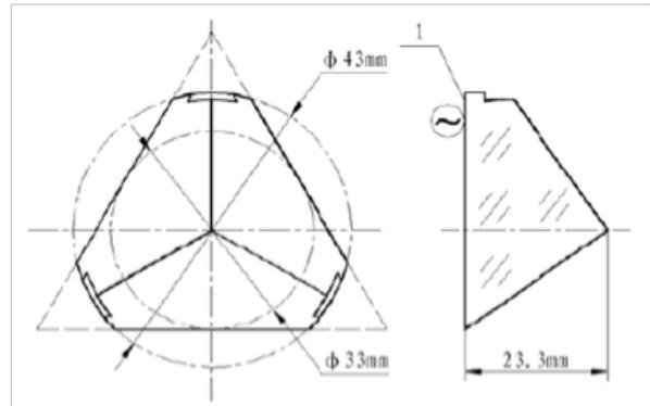
Figure 9-5. (Left) Galileo-IOV CCR tested at LNF. (Right) Drawing of the CCR.
