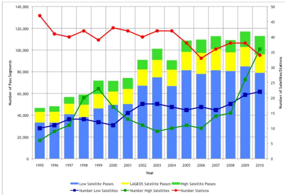
Figure 3-5. Network data yield continues to increase with the reopening of stations after repair and upgrading, improved network proficiency, and additional satellites mainly at GNSS altitude.
