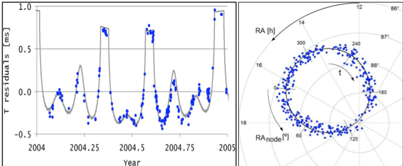
Figure 12-28/Left: Ajisai spin period residuals (blue dots) and the model function (grey line) which depends on TSI (Total Solar Irradiance) acting on Ajisai; plotted for the year 2004.
