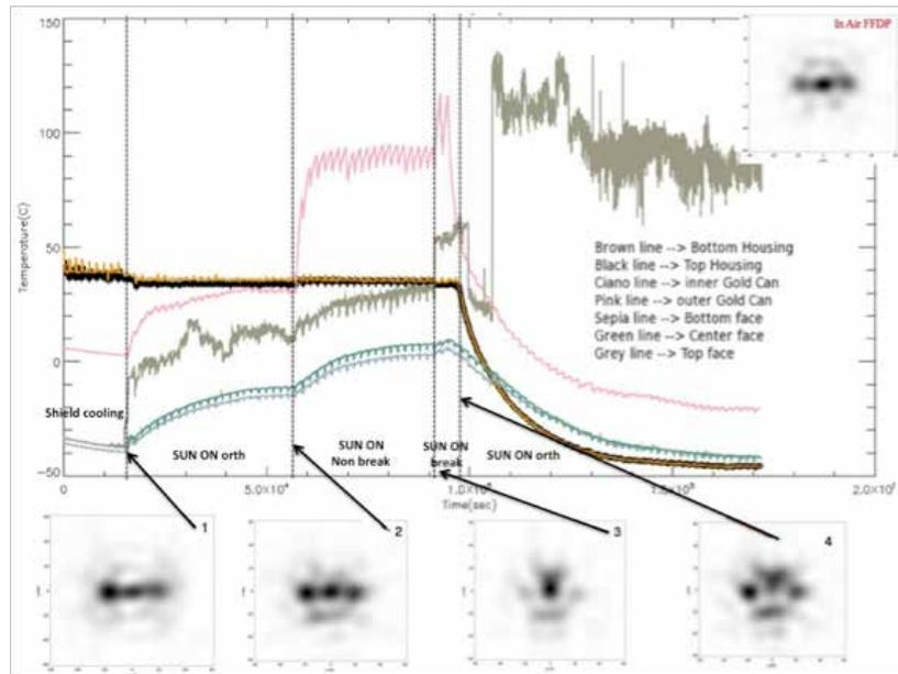
Figure 9-8. Temperature variations of the housing parts and relative FFDP
