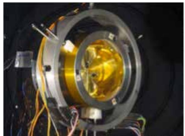
Figure 9-7. MoonLIGHT CCR inside the SCF cryostat
