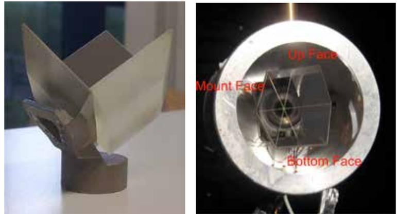
Figure 9-3. The NASA-GSFC hollow retroreflector. (right) CCR in its test configuration
