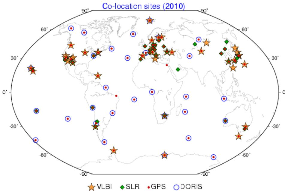
Figure 3-10. Current status of SLR, VLBI, DORIS, and GNSS co-locations (2010).
