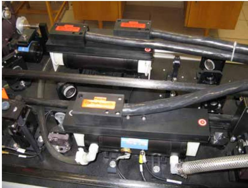
*Figure 12-14. After 20 years, these laser heads do not properly function; the reflective cover inside is destroyed and it is dangerous for other laser elements.*
