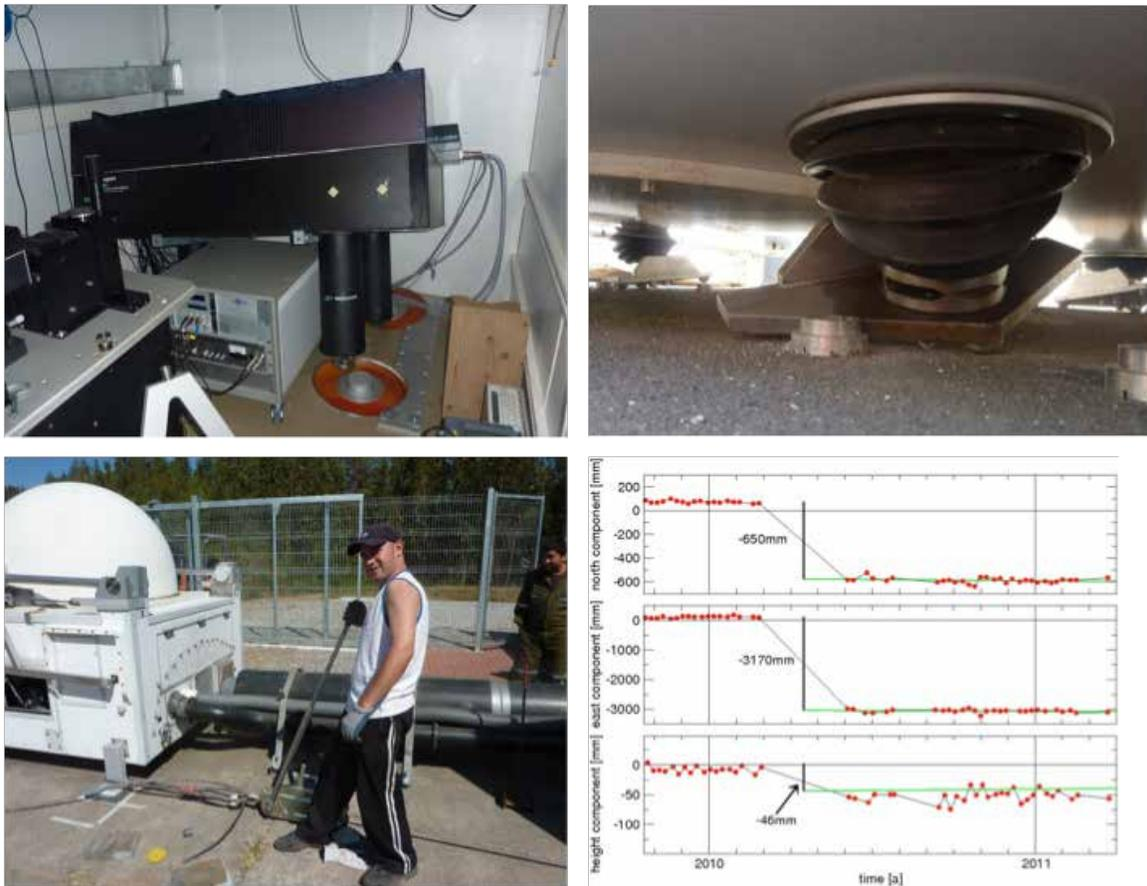
Figure 12-19: Photos taken after the earthquake of February 27, 2010. Upper left and right: Telescope and optics table overthrown by the shocks of the earthquake. Lower left: Coarse re-alignment of the telescope. Lower right: Displacement due to earthquake measured by TIGO-SLR.
