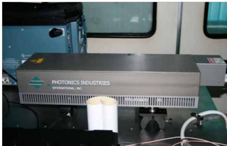
*Figure 12-16. The photo of RG30-L-532 laser*
