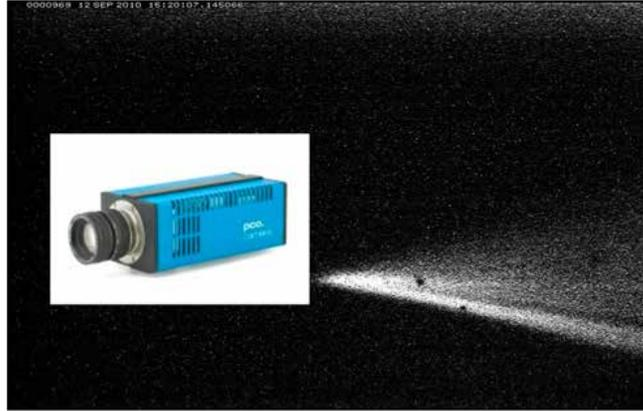
Figure 12-17. The PCO-1600 camera and laser beam imaging in daylight.
