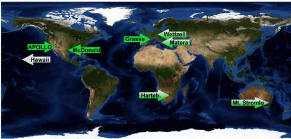
Figure 3-4. ILRS sites with potential lunar capability demonstrated in the past or planned for the near future. The green arrows indicate active stations, the green-grey arrows the possible future stations and the grey arrows the former stations
