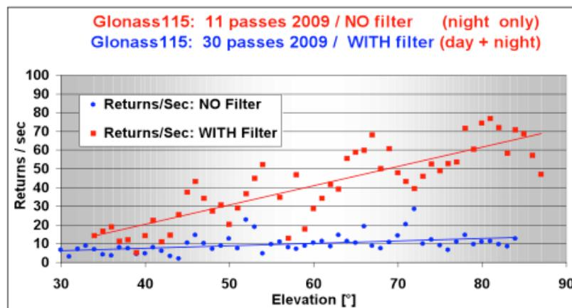
Figure 12-27: Increase of returns for distant satellites: 3 times more returns when filter is removed during night
