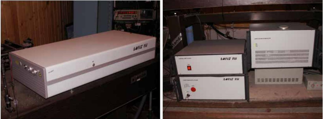
Figure 12-54. The new laser system of our station, installed in 2008. The laser unit (left) and power supply, control unit, laser cooling unit (right).
