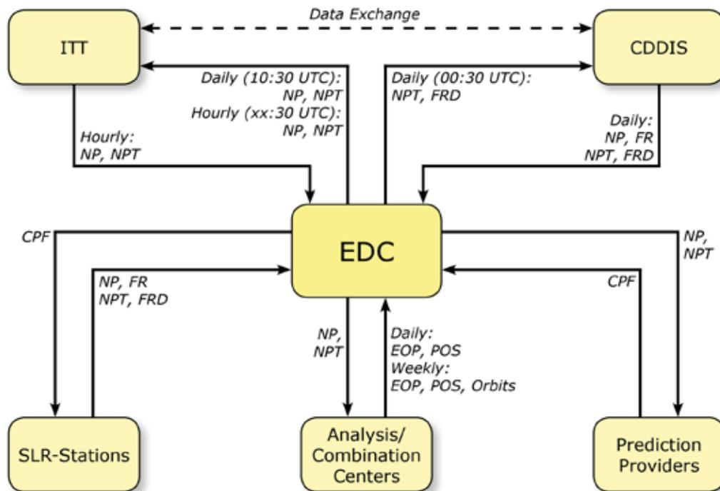
Figure 5-3: Data Flow of EDC within the ILRS
