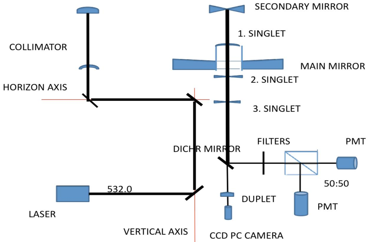
Figure 12-69. Laser telescope channels separation principle (not in scale)
