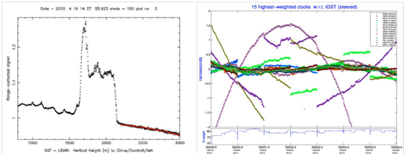
Figure 12-44. (left) A LiDAR backscatter profile through the atmosphere containing some volcanic ash.
