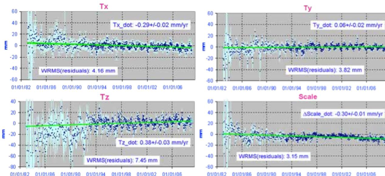
Figure 6-1: Time-series of X, Y, and Z offsets and scale factor of the ILRS-A official combination origin with respect to the reference ITRF (SLRF2005) origin (proxy for “geocenter” variations) and scale as observed by SLR (1983.0 – 2009.0).
