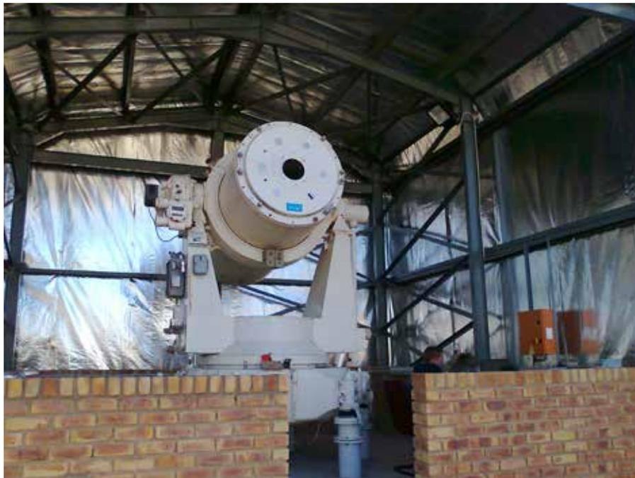
*Figure 12-40. The SLR/LLR telescope located in its newly built enclosure. This enclosure runs on three tracks. Adjacent to the enclosure is a modified 12-meter long shipping container which will house the control room, laser system and power supplies. It is planned to move the new SLR/LLR system to the semi-arid Karoo region, to a site close to Matjiesfontein where we are developing a new space geodesy and geophysics observatory.*
