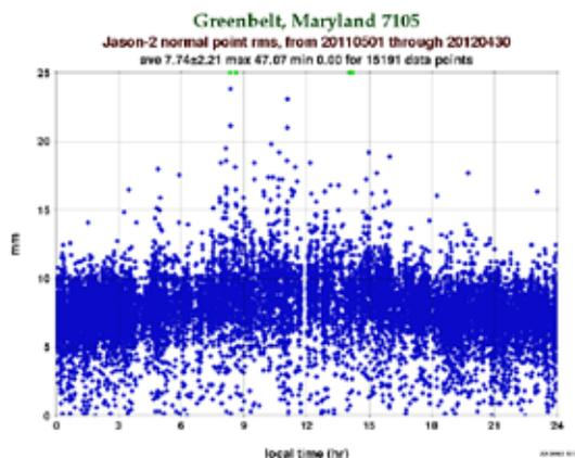
Figure 7-7a. Jason-2 normal point RMS at Goddard MOB LAS-7 (as a function of local time) for the past year
