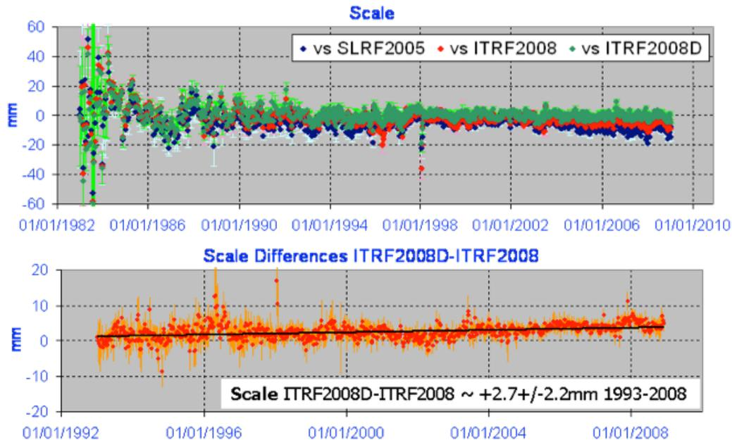
Figure 6-2: Time-series of scale factor variations as observed by SLR (1983.0 – 2009.0) compared to the two candidate ITRF2008 combinations. Note that there is no longer a trend on the SLR scale, especially when compared to ITRF2008D. The two candidate solutions differ by 0.4 ppb/y over 1993-2008.
