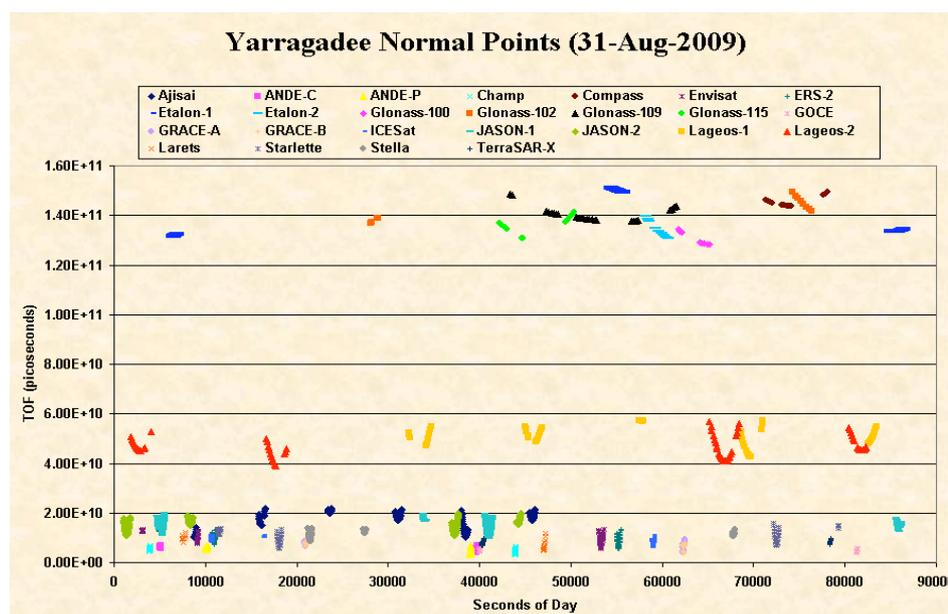
**Figure 2** Interleaving of satellite tracking at Yarragadee in one 24-hour period
