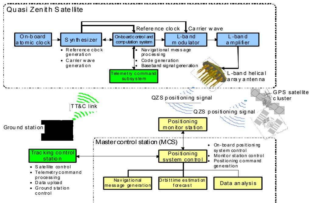
Fig.1.3-1 Configuration of the QZSS system
