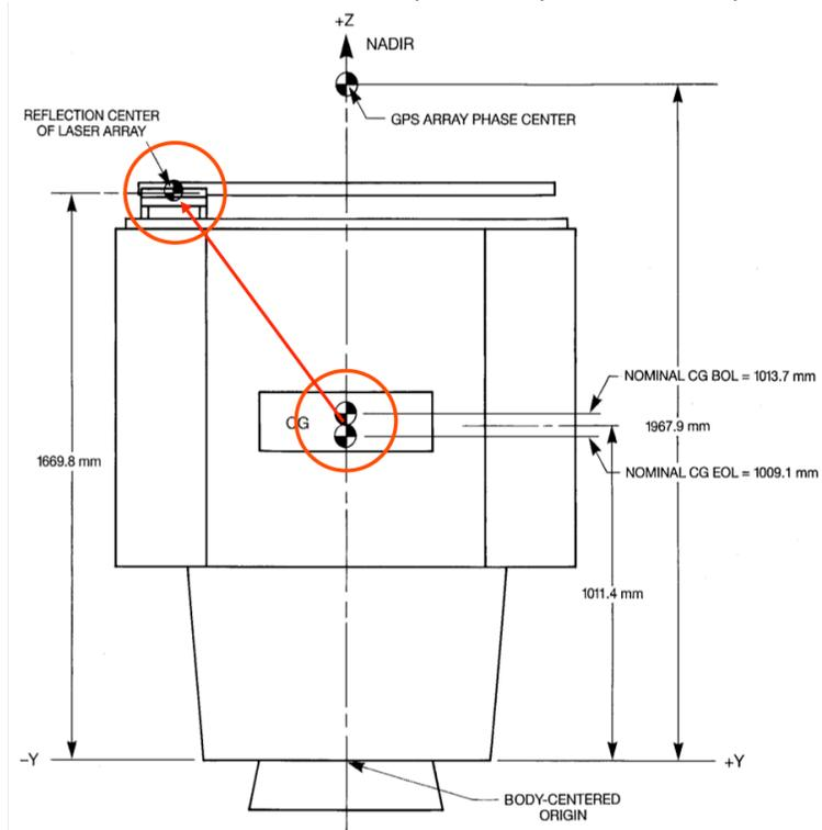
**Figure 2.** XY-plane view of the GPS s/c illustrating the locations of the GPS satellite center of gravity (CG), the effective laser array center of reflection, and the phase center of the L-band transmitting antenna array. The positive-Z coordinate axis is in the direction of satellite nadir.
