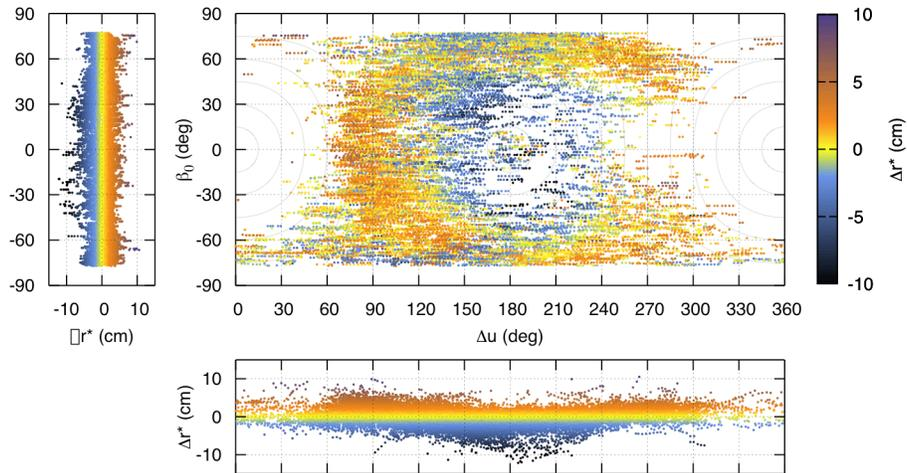
**Figure 5.** Color-coded de-meant SLR range residuals determined using the ROCK SRP model [Fliegel *et al.*, 1992]. The residuals are projected into a coordinate system where  $\beta$  is the elevation above Sun above the satellite's orbital plane and  $u$  is the argument of latitude of the satellite relative to that of the Sun. After Flohrer [2008].
