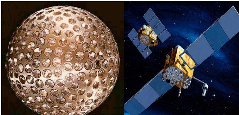
**Figure 3.** LAGEOS spacecraft and a pair of typical GPS spacecraft.
