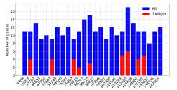
Figure 1: Bar plot showing the share of all passes (blue) of the chaser object per event which can be tracked with debris laser ranging by the Graz SLR station (red). The x-axis lists individual close approach events with their IDs.
