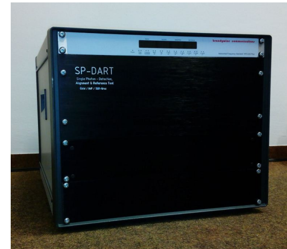
Graz SP-DART electronics box with GPS T&F receiver, Riga USB-ET, FPGA, ...
