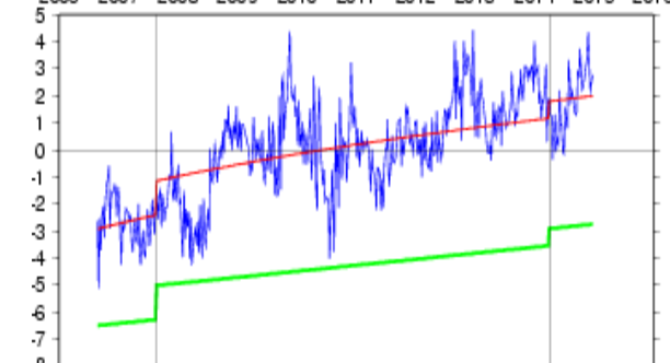
Trajectory: Blue: Raw, Green: Linear, Red: PSD model Vertical gray lines represent discontinuities
