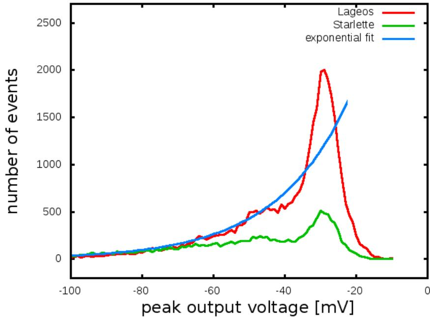
**Figure 1.** Histogram over the accumulated signal returns over several month of data of the peak output voltage of a micro channel plate receiver, installed at the Wettzell Laser Ranging System.
