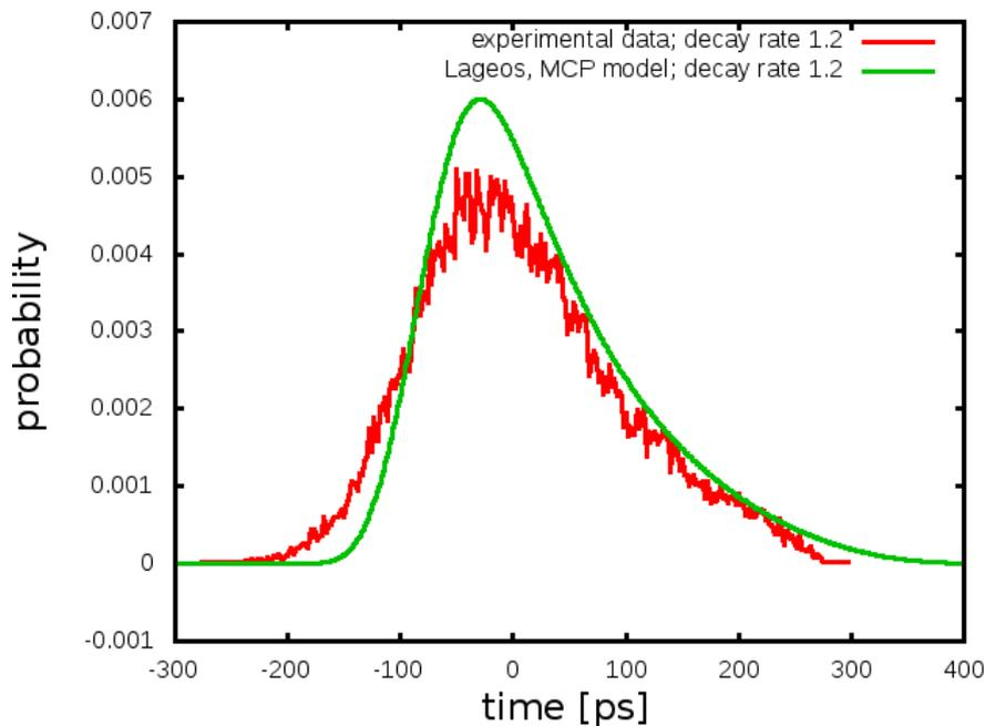
**Figure 5.** Residual histogram of accumulated data of distance measurements to LAGEOS satellite passages, performed at the Wettzell Laser Ranging System with our theoretical model (green) of the satellite response.
