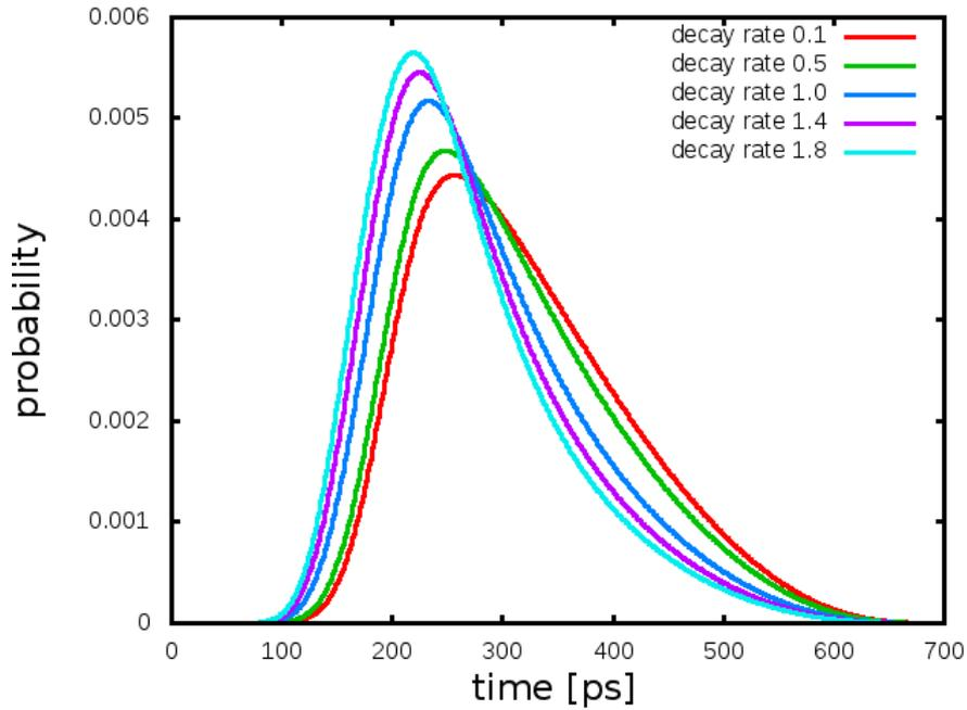
**Figure 3.** Residual histogram, derived from a convolution of our micro channel plate receiver model with the satellite signature of a LAGEOS satellite in the mixed state for different decay rates in the seeding photoelectron statistics.
