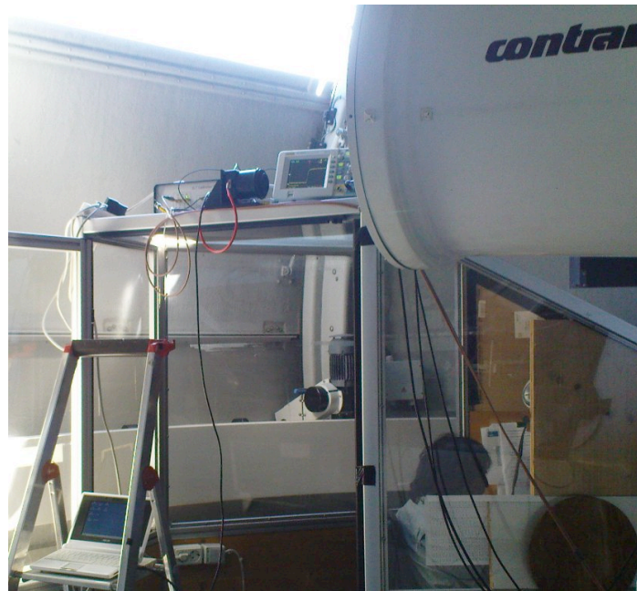
Figure 2. ELT Calibration Device installed in a dome in front of the Graz SLR system. SLR system telescope (right top), ELT detector (black, top center), ELT calibration Timing (top, left), process control and data acquisition PC (low left).
