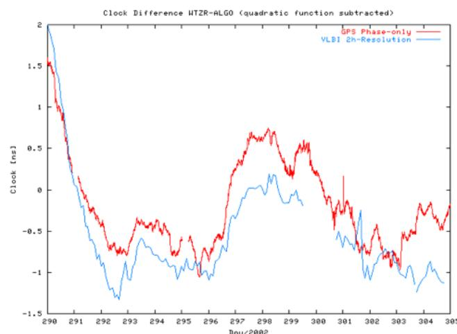
Figure 1: Illustration of variable system delays between VLBI and GNSS
