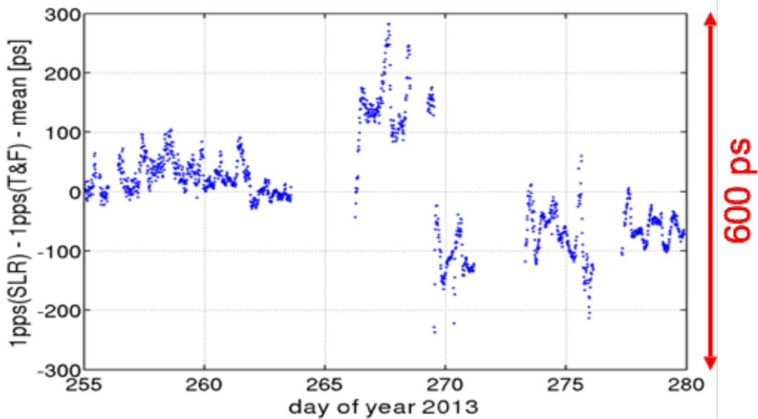
Figure 2: Variations in the time delay between the Cs master clock in one building and the SLR system in another building.
