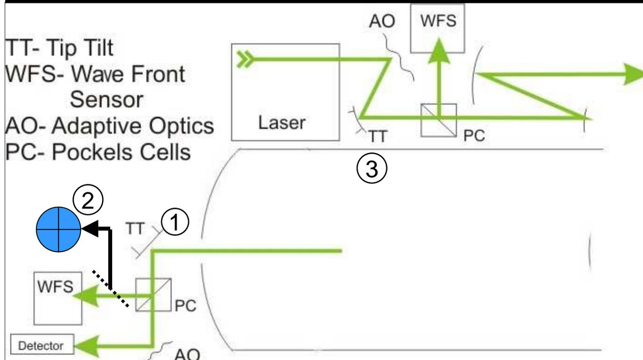
1. Tip-tilt mirror to actively fine-adjust pointing to retro-reflector
