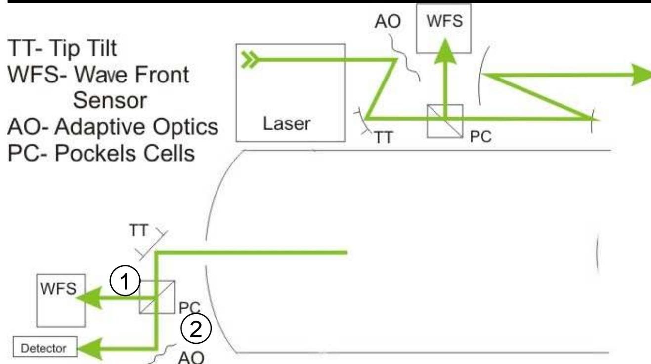
1. **Time-gated detection of wave front through main telescope**
