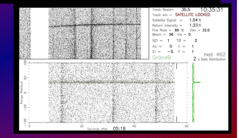
However, the ISA card needs feedback from the laser which we are unable to provide so instead we change the firing rate of the laser in real time through software.
