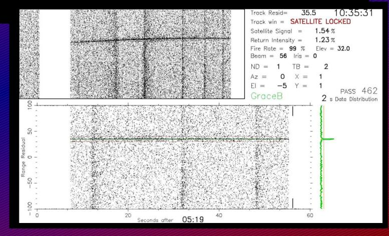
A clash is easily foreseen because the laser firing is predictable. So the software finds a firing rate without clashes. However this is limited to step changes of 10 Hz on
