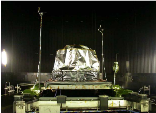
Thermal Vacuum Test of L-band Antenna Engineering Model (February 2007) [JAXA]
