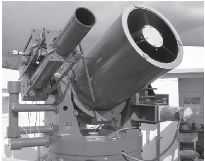
Figure B-6. The Borowiec SLR mount.
